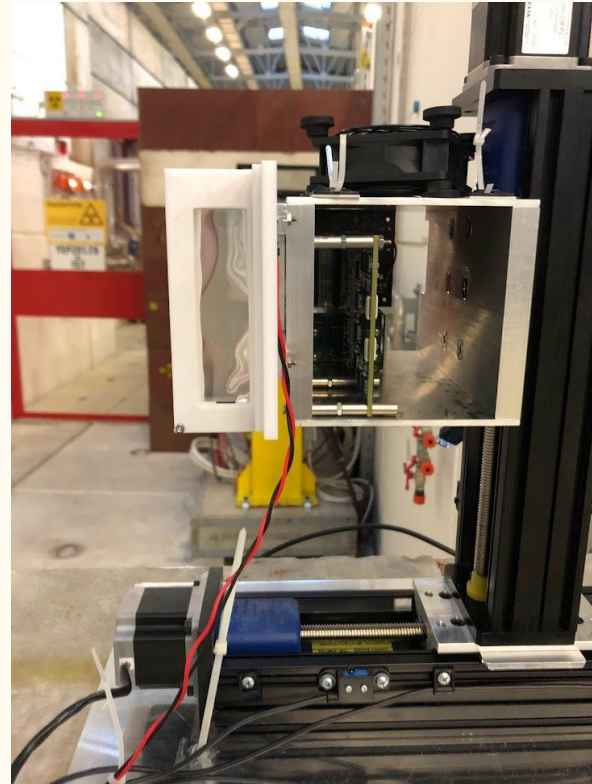
TS 12 bar setup at the T9 testbeam. Note that Slide 1 in Back Up has more run details.
