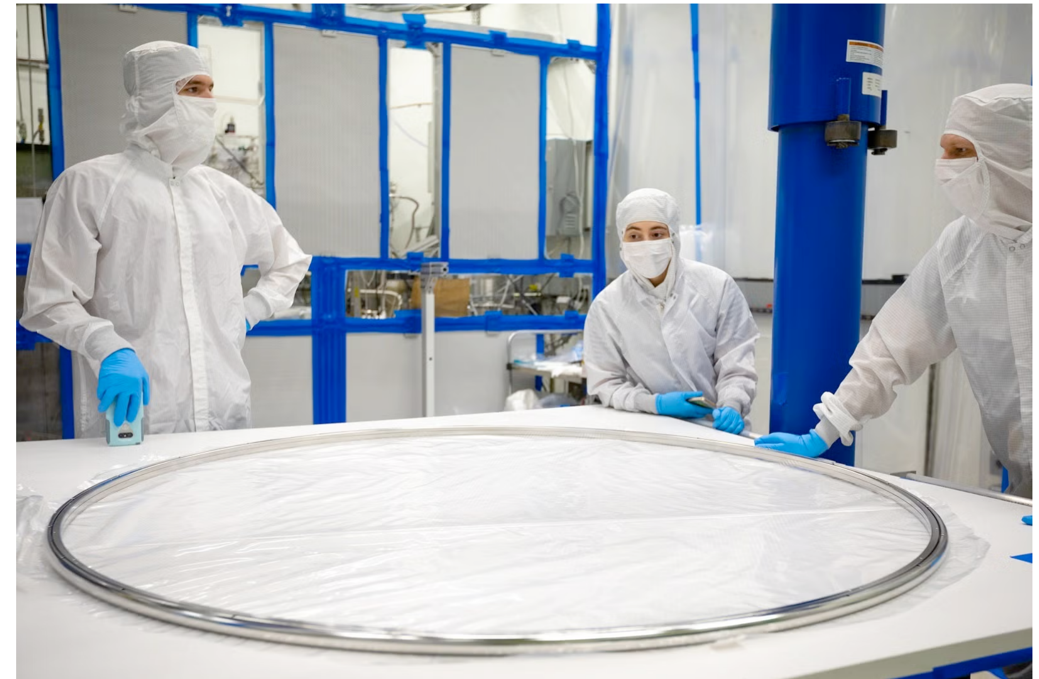
LZ electrode, treated to prevent emission
